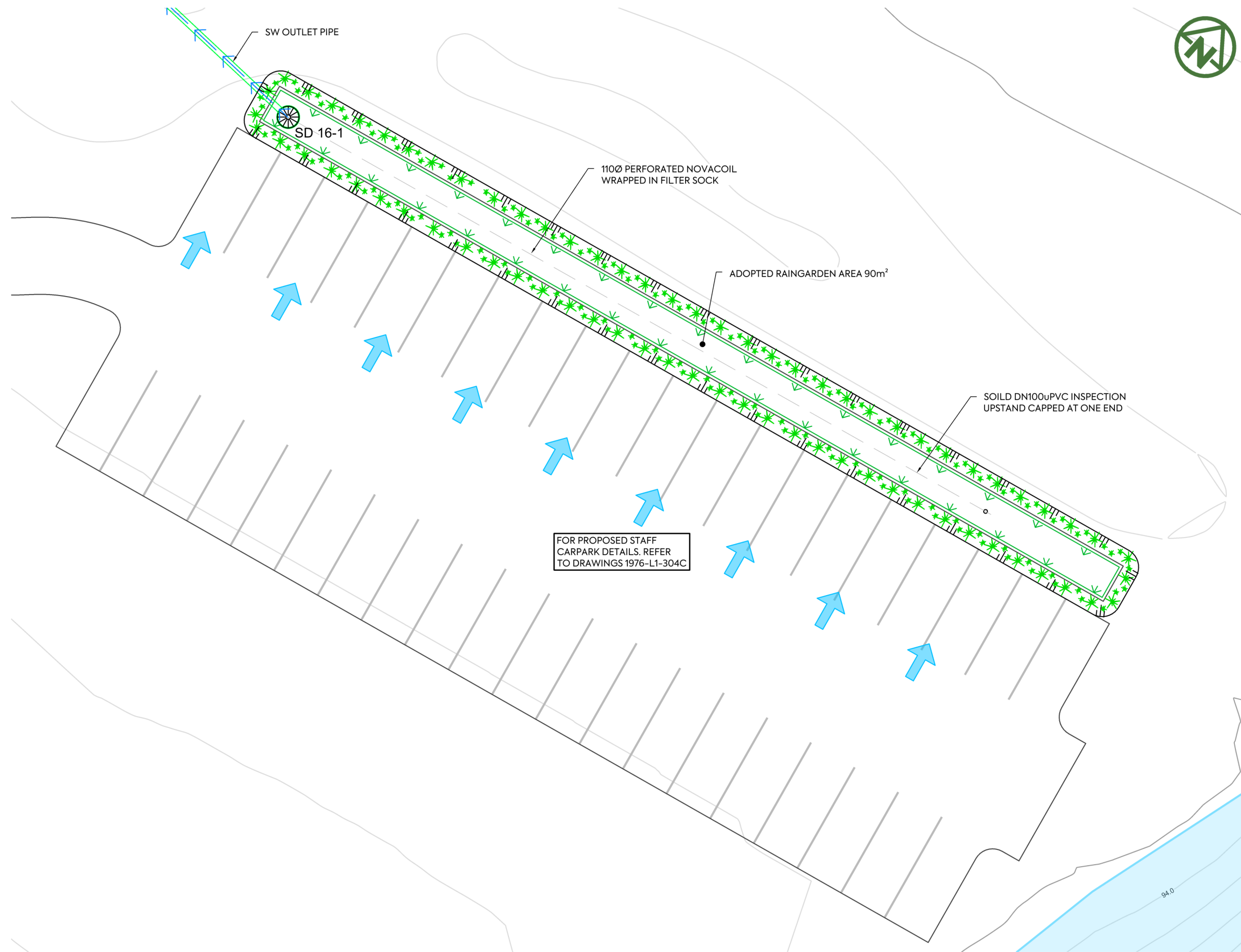
PLAN VIEW - STAFF CARPARK TREATMENT (OFFLINE RAINGARDEN RG2) SCALE: 1:200 @ A3
